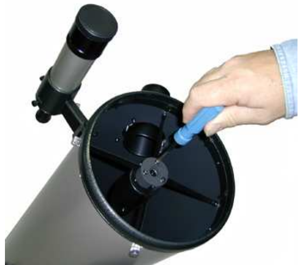
Figure 13 Adjust the tilt of the secondary mirror by adjusting the three alignment screws with a Phillips head screwdriver
