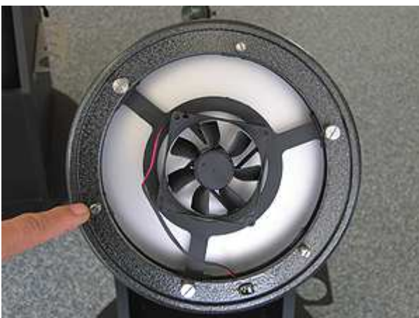
Shows the Primary Mirror locking screws
